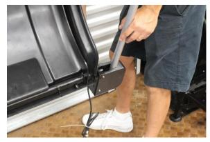
Rout the "B-Gauge" cord through the nylon straps and plug it in on the side of the WB55 chassis. Tighten the nylon straps.
