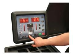
"D" (diameter of the wheel in inches; Use caliper, or refer to marking on tire)
