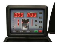
STEP 10: When the cycle is finished, the display will read "Add 3.50" (100 grams). Remove the calibration weight from the inside edge of the wheel. Rotate the wheel until all the outside weight indicators are fully lighted. Apply the 3.5 ounce (100 gram) calibration weight to the outside edge of the wheel at the 12 o' clock position. Lower the hood and spin the wheel.
