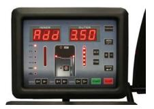
STEP 11: After the cycle is finished, the screen will flash "EEP ON" then return to "000 000". Your balancer is now calibrated.
