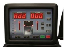
STEP 9: When the cycle is finished and the tire stops, the display will read "3.50 Add" (100 grams). Rotate the wheel until all the inside weight indicators are fully lighted. Apply the 3.5 ounce (100 gram) calibration weight on the inside edge of the wheel at the 12 o' clock position. Lower the hood and spin the wheel.
