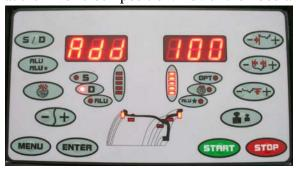
**STEP 11:** After the cycle is finished, the screen will flash "**EEP ON**" then return to "**000 000**". Your balancer is now calibrated. To check the calibration, rotate the wheel so that the weight is positioned at 6 o'clock. All of the weight indicators should be fully lighted as shown below.
