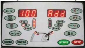
STEP 10: When the cycle is finished, the display will read "Add 100" (3.5 ounce). Remove the calibration weight from the inside edge of the wheel. Rotate the wheel until all the outside weight indicators are fully lighted. Apply the 100 gram (3.5 ounce) calibration weight to the outside edge of the wheel at the 12 o' clock position. Lower the hood and spin the wheel.
