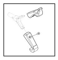
C103000013 Nylon demounting head C103000014 Nylon mounting head 0207023 Screw M8X20 (Nr.2)
