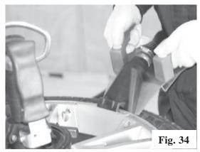
• Continue to inflate the tire with short jets of air by depressing the inflation pedal and constantly check the pressure between air jets until the required pressure has been reached.
