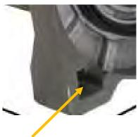
Make sure not to bottom the bolt against the mounting flange.
