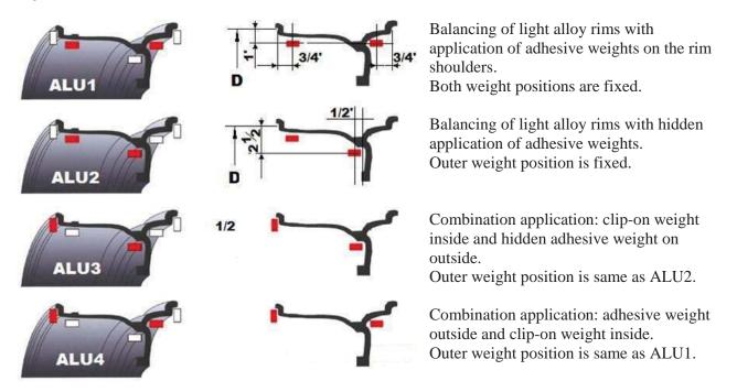
Hidden adhesive weights can be applied by the pusher on the automatic gauge, as shown in the figure 17.
