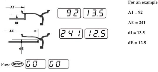
After performing the balancing spin, pull the gauge to the inner and outer position separately until "0" is shown on the digital readouts, where to apply the adhesive weights
