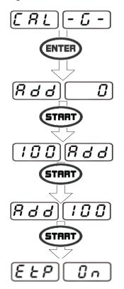
Mount a wheel with average data on the shaft. Entry the exact data of the wheel mounted.
