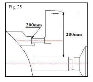
When making the "D" calibration, make sure that 200mm is measured from the shaft surface where is with the maximum diameter.
