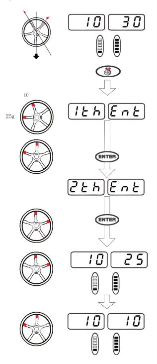
At ALU  $\stackrel{\wedge}{\succ}$  mode, the unbalanced amount of the outer side of the rim shown on the digital readouts is 30g.
