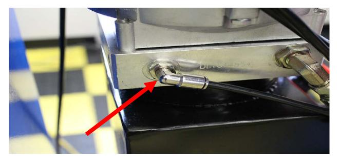
This is an option and is not necessary for your lift to function properly. Atlas cylinders and seal are manufactured to exact tolerances. In the unlikely event that a leak were to develop in the cylinder cup seal, the hydraulic fluid leaking past that seal would drip on the floor. This optional line (if installed) would trap any fluid leaking past the cup seal and return leaked oil to the fluid reservoir.
