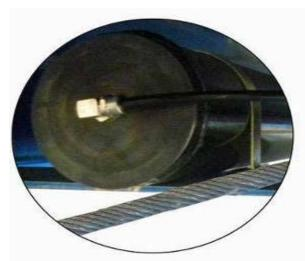
The installation guide for the 412/412A, 414/414A, 408-SL or the 409-HP shows how to connect a 90 degree fitting and plastic line/hose to the rear of the cylinder. This line is then connected to the Power Unit (see below).
