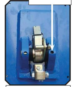
Use M10 x 20 Hex Head Bolts to secure the pulley bracket
