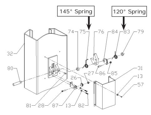
Fig. 25 Offside safety device
