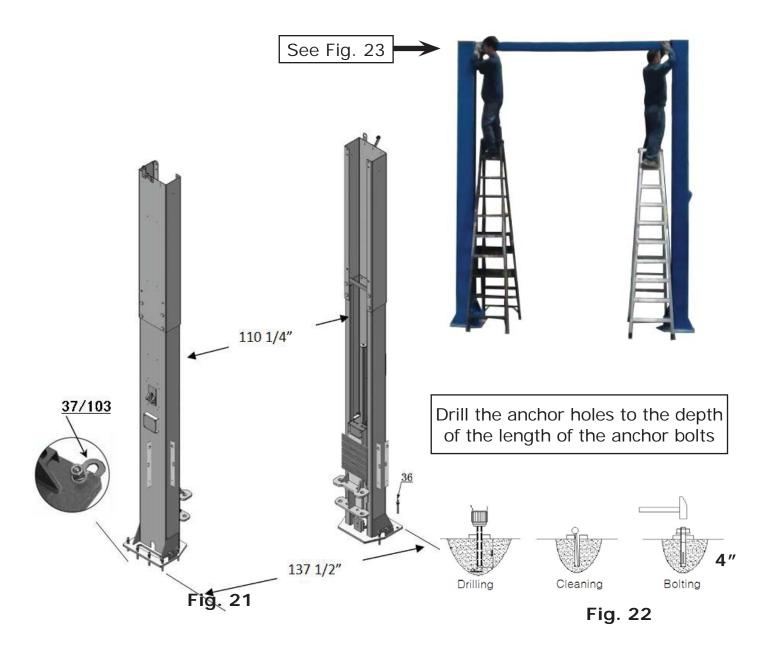
Install the anchor bolts. Check the posts for plumb with level bar, and adjust with the horseshoe shims if the columns are not plumb. Do not tighten the anchor bolts.
