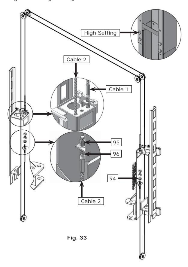
2. Low setting cable connection. For a ceiling height between 4250mm (167 3/8") and 4350mm (171 1/4").
