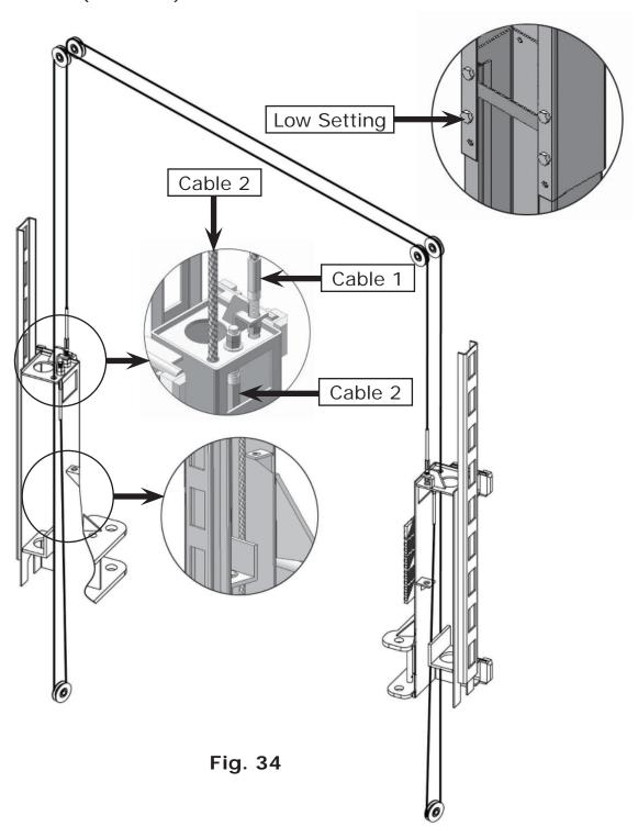
3. **Special low setting cable connection PV10PX.** For a ceiling height between 3820mm (150 3/8") to 4250mm (167 3/8"). This setting requires the optional short cables.
