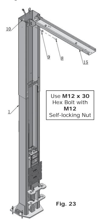
2. Assemble overhead top beam and tighten the anchor bolts.
