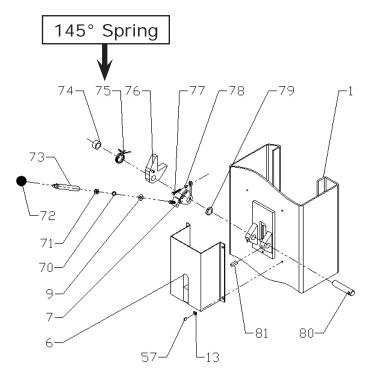
Fig. 26 - Power side safety device
