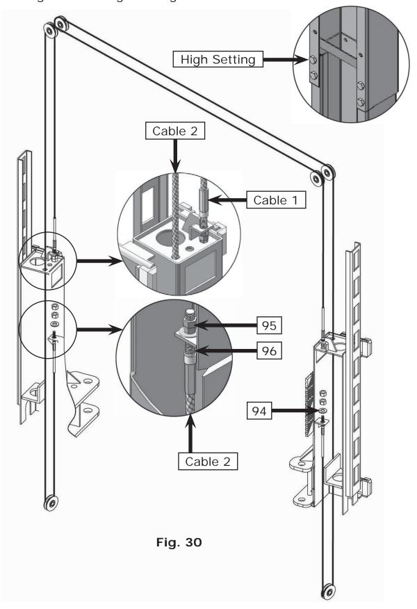
2. Low setting cable connection. For a ceiling height less than 3750mm (147 5/8")
