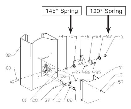
Fig. 27 - Offside safety device
