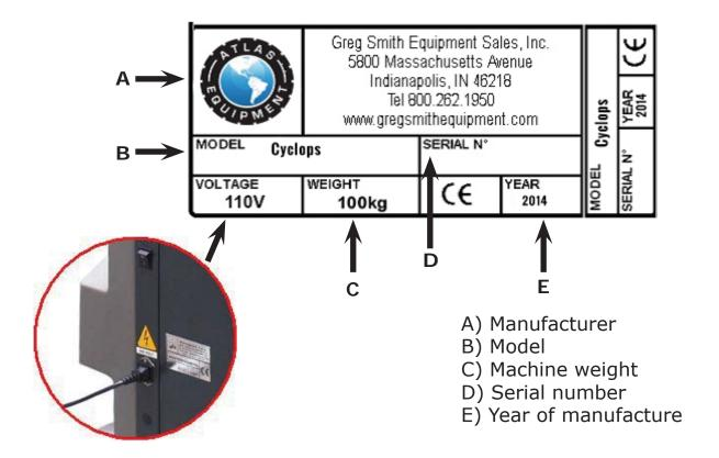
WARNING: It is strictly forbidden to tamper with, alter, or even remove machine identification plate; do not cover it with temporary panels, etc... as it shall always be clearly visible.
