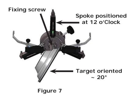
Mount targets onto wheel clamps at an angle of approximately 20° and fit them to the vehicle. Make sure that wheel clamps are secured in place with the spokes positioned strictly vertically (12 o'clock), as shown in Figure 7.
