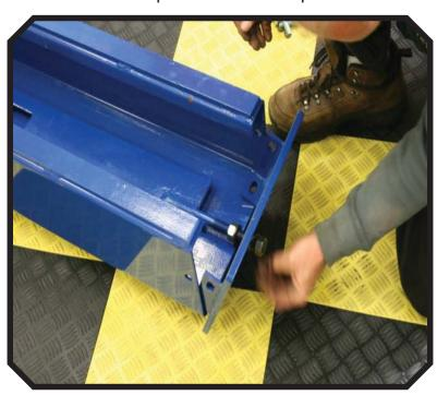
8. Maneuver the rear crossbeam into each column. Screw the wear blocks to the rear cross beam: 12 pan head screws supplied.
