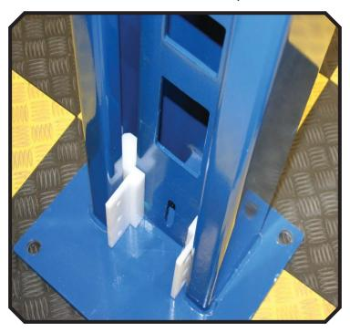
5. Using the bolt supplied at the bottom of the column, attach the short lock ladders. *Do not tighten the bolt*.
