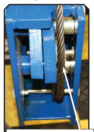
Note: The position of the equalizing cable is in front of the *small white* safety lock pulley. *Front cross beams.*
