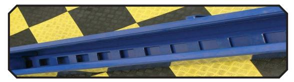
3. Insert white wear blocks into the front cross beams' carriages. There are 4 white wear blocks per side. Make sure the rounded edge of the white wear block is facing outward. The rounded edge makes contact with the inside corners of the column.
