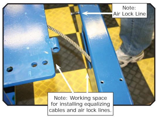
3. Route each equalizing cable into their positions. The longest cable is the Passenger front (421.4"). The 2nd long cable is the driver's front (359.3"). The 3rd long cable is the passenger rear (218.2"). Shortest cable is the driver's rear (156.1").
