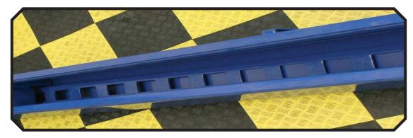
3. Insert the **short locking ladders** into the rear columns. Set the columns upright into their relative positions.
