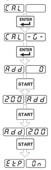
Mount a wheel with average data on the shaft. Entry the exact data of the wheel mounted.
