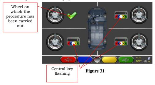
On Figure 31 the front left wheel is shown with a tick on the side, to indicate that the procedure has been carried out on that wheel. Procedure can anyway be repeated by pressing again the central key of the concerned detector. When the Run-Out procedure has been completed on all wheels, programme will automatically go to the next phase.
