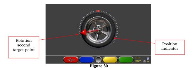
Turn wheel by 240° and, once the target position is reached, press detector keypad central key, as indicated on the screen Figure 28.
